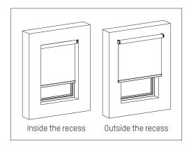
This can be done inside the recess or outside the recess. If you install the blind outside the recess, it is mounted on the wall and will be placed over the window with overlap on both sides.
