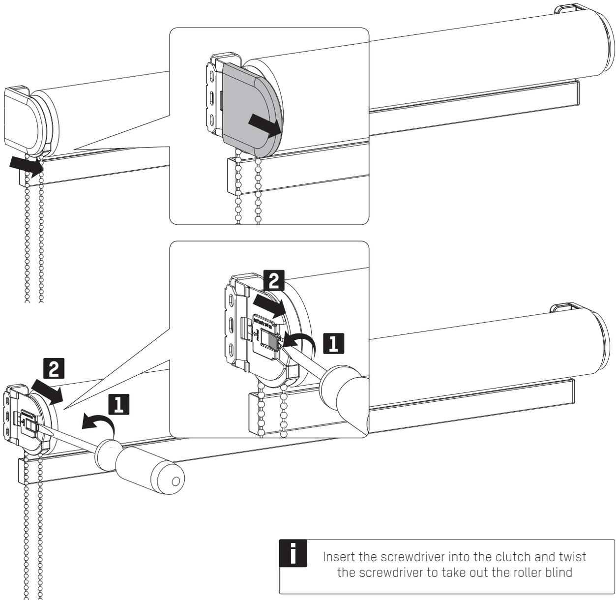
**i** Insert the screwdriver into the clutch and twist the screwdriver to take out the roller blind
